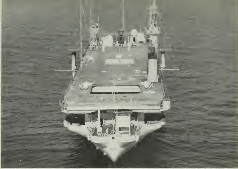
DECKED OUT —Ex-Navy carrier USNS Croatan is being operated by MSTs for the National Aeronautics and Space Administration to gather information on atmosphere and ionosphere as relayed from missiles fired off ship's stern.
